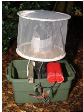
Figure 1-6 - CDC gravid trap Source: Perich and Gleiser, 2003
