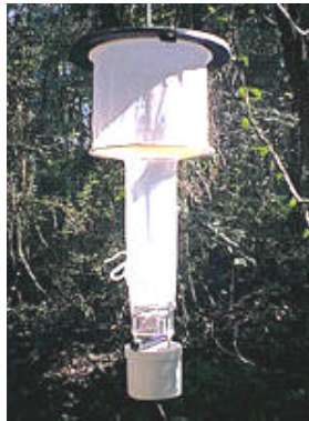
Figure 1-3 - The miniature CDC updraft blacklight trap From John W. Hock Company (johnwhockco.com)
